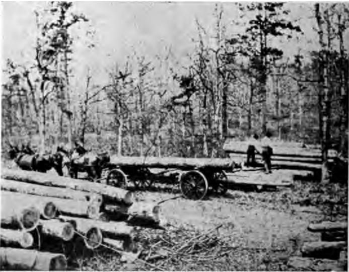
FIG. 48. — A Four-wheeled Log Wagon at the Skidway. Missouri.
